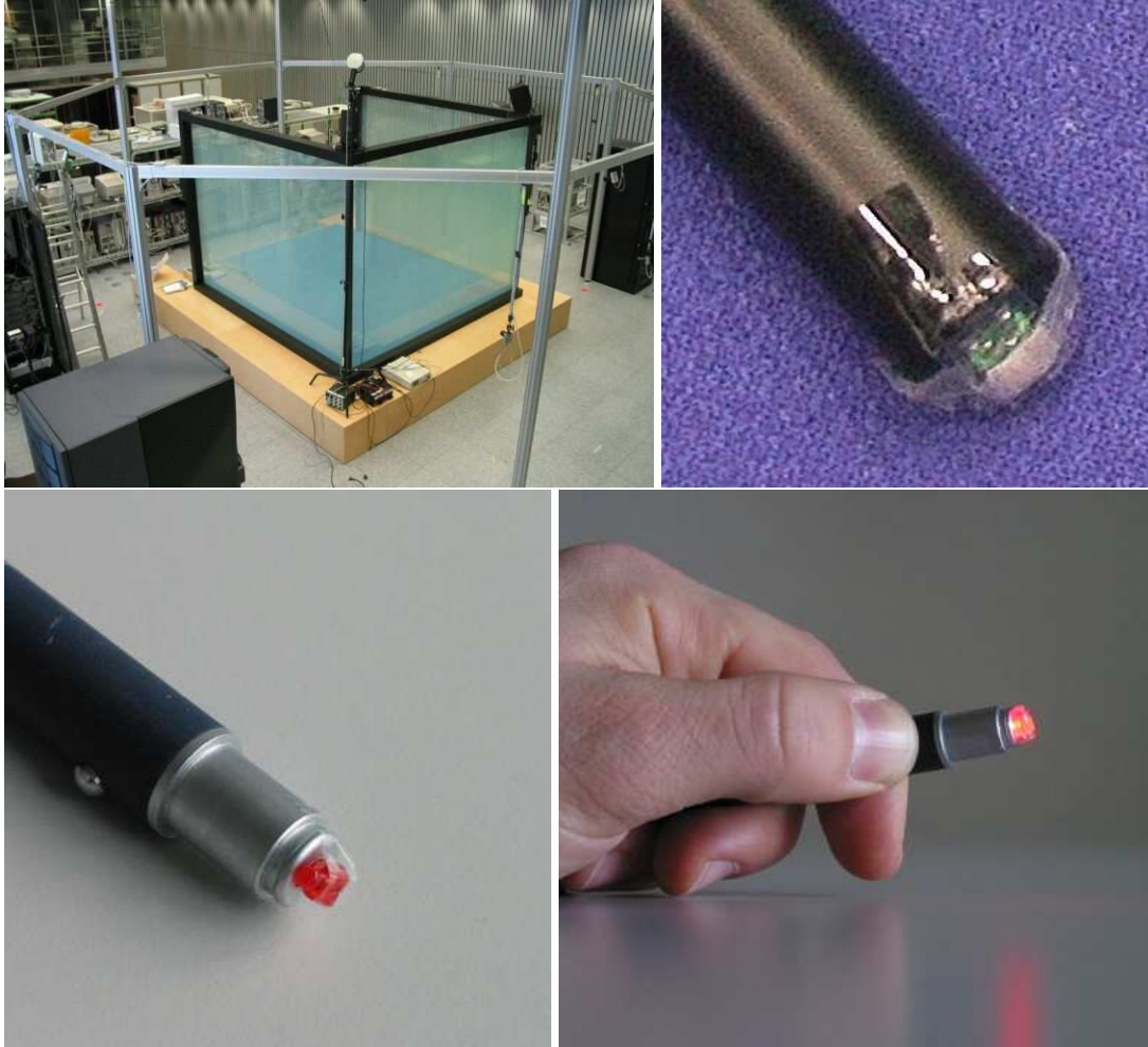
Figure 2: Immersive virtual environment BlueC [10] and our modification of a laser pointer. A small piece of transparent green or red plastic is attached to the laser pointer. The modification has been invented in order to get better visibility from different viewpoints. However primitive a solution it is, it does the job very well. The working volume is inside the glass CAVE. Four cameras are mounted on the top four corners of the construction and the remaining 12 cameras are mounted on the aluminum scaffold that encompasses the CAVE.
