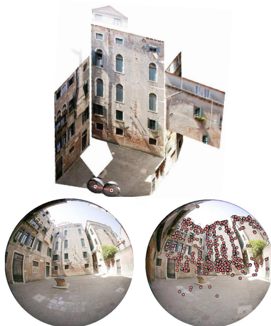
Fig. 1. 3D metric reconstruction of a Venice yard from two uncalibrated omnidirectional images with automatically detected point correspondences.
