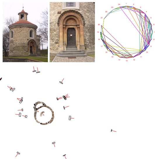
Figure 1. Reconstruction from a wide base-line scenario after Euclidean BA: the St. Martin rotunda on 24 images, 89% data missing, top view. Some cameras are positioned very close to each other while some are distant making the SFM problem difficult
