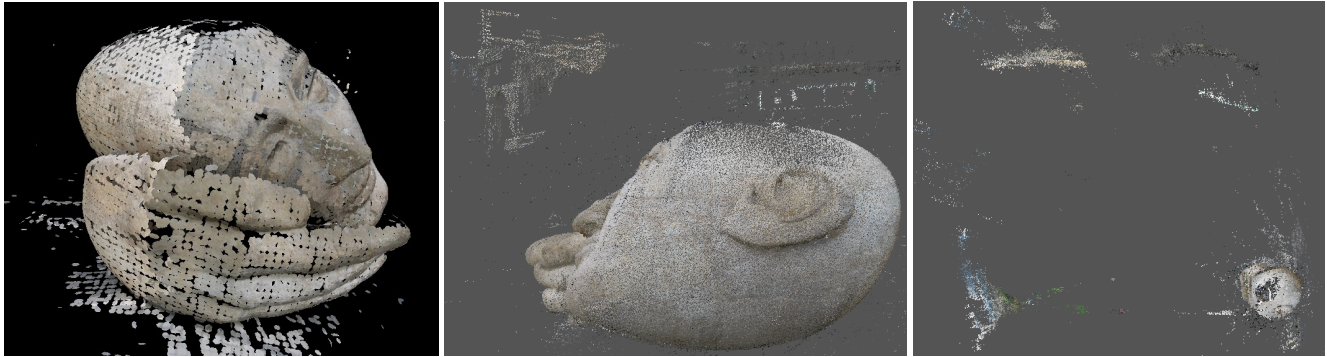
Figure 6: All-around reconstruction of the Head statue (from left): front view using fish-scales, side and overall top views with reconstructed buildings around using point clouds (10% points shown)
