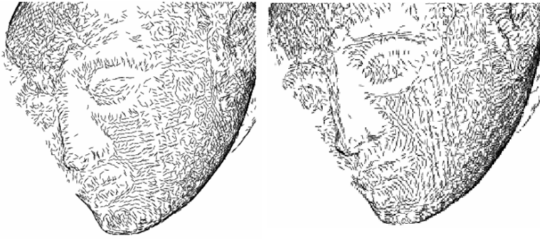
Fig. 6. Geometry Pipeline Output: The two curvature lines foliations extracted on a 2D component in the cloud from Figure 7
