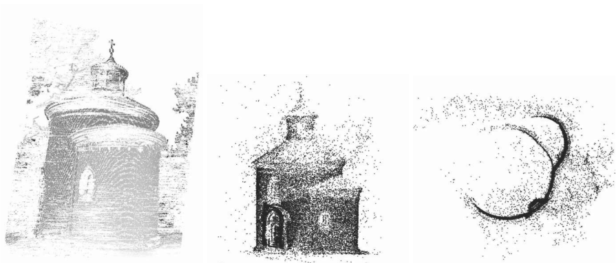
Fig. 4. The disparity map for the first two images in the second row in Fig. 2 and Point clouds for the St. Martin scene (a front and a top view). Only 2% of all points are shown
