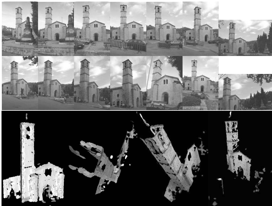
Fig. 7. Input images and the fish-scale model for the Valbonne scene. Note that the walls of the tower are mutually perpendicular
